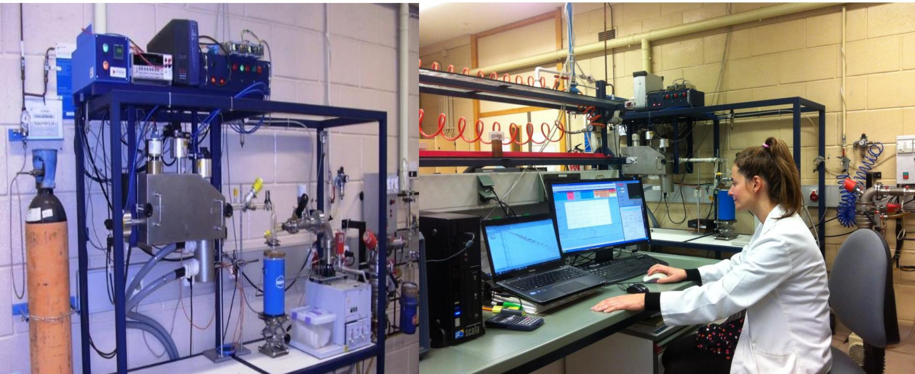
Two MKS Baratron Capacitance Manometers 631A (Calibrated NIST)
